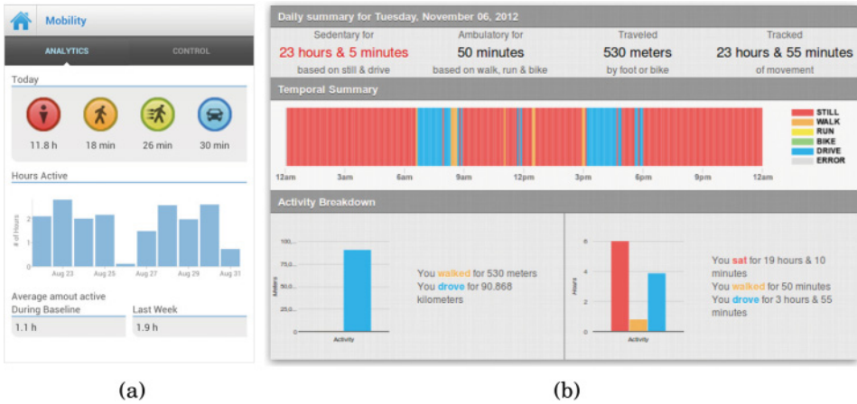
Fig. 3. Mobility. (a) The app analytics screen showing mobility and ambulatory summaries for 1 and 10 days. (b) The Web-based Mobility Dashboard showing a daily summary of the user's mobility status, mobility times series, and activity breakdown based on time and distance.
