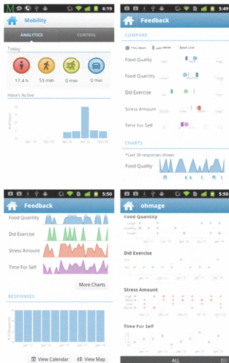
Figure 2. Snapshots of feedback graphics available in the ohmage Android application. Summaries and plots of general mobility states (still, walk, run, drive) captured from the continuous actigraphy trace (top left); graphic comparing baseline responses with responses from current week and past week self-report measures (top right); sparkline time-series and higher resolution time-series plots of various self-report measures (bottom left and right, respectively).
